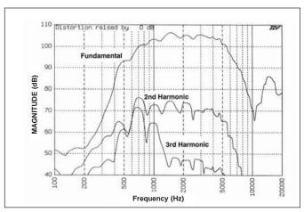
SC-15 (8 Ohm Model) (Harmonic Distortion 1watt at 1 meter)
